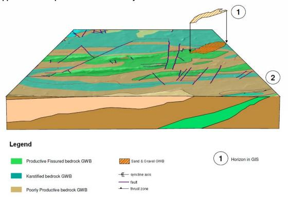
$<sup>^{\</sup>star}$  Note, in this example, the unconfined and confined components of the bedrock aquifers are considered to be part of Horizon 2
