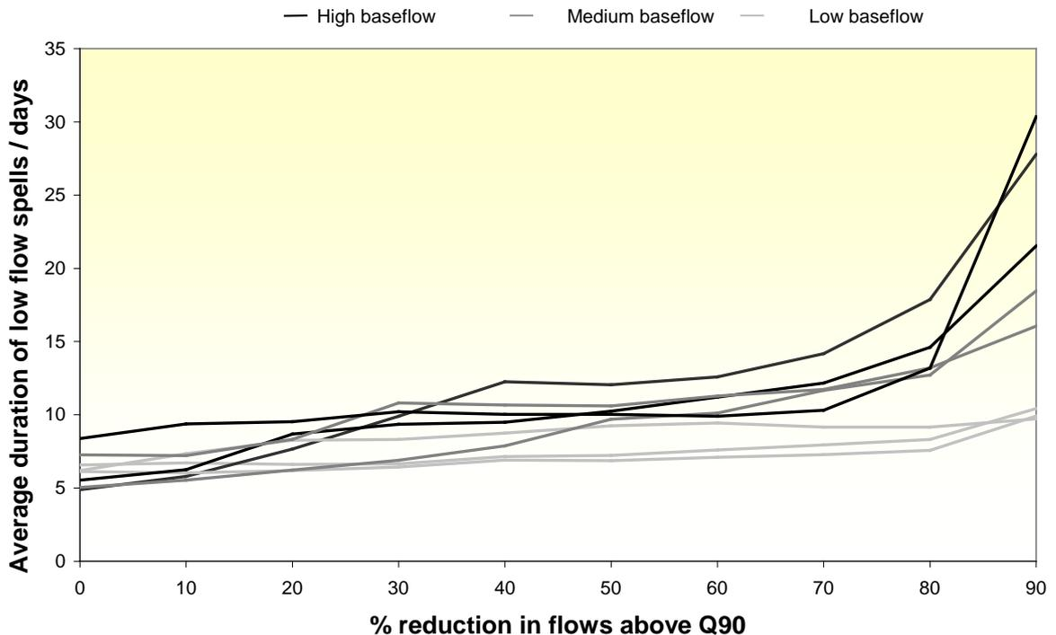
**Figure 2. The increase in mean duration of low flow spells (flows < Q90) with percentage reduction in flows above Q90 for 8 SEPA gauging station records. Stations are grouped by baseflow index (BFI) where low is <0.35, medium is 0.35 to 0.45 and high is > 0.45**
