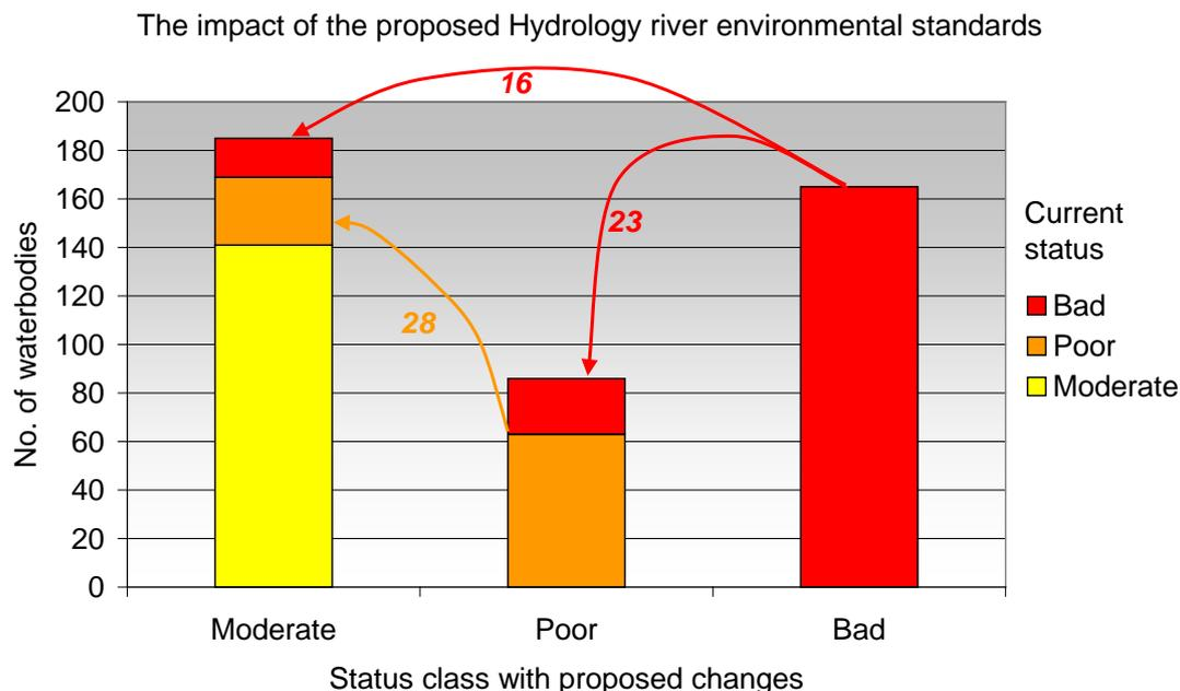
**Figure 5. The impact of the proposed changes to high/medium flow hydrology environmental standards to Scotland's 2009 hydrology classification. Note: there are no changes on waterbodies currently classified as High or Good**
