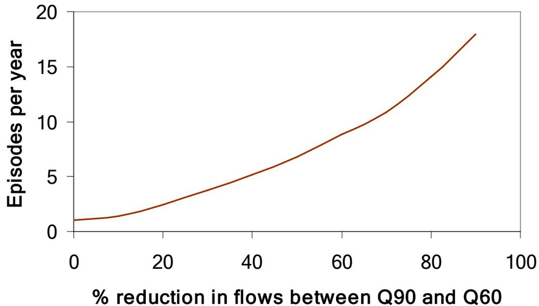
**Figure 3** The impact of a reduction in mid range flows upon the number of low flow episodes. The curve represents the mean of 8 sites. A low flow episode is taken as an event where the duration equals or exceeds the duration of a natural low flow event with a 1 year return period.
