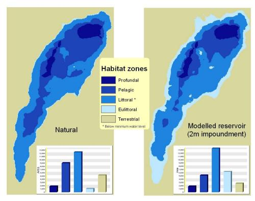
Figure 3 A visualisation of habitat zones for Lochindorb under natural (left) and impounded conditions (right). Note; the bar charts show the relative areas of each zone. Note: the modelled impoundment of Lochindorb is used to demonstrate the impact on habitat zones and does not reflect current or proposed conditions in the loch.
